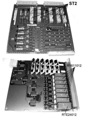
Fig. 1. PCB boards of MRPD with output electromechanical relays of different types
